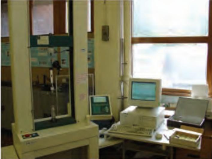
Figure 5 - Hounsfield Universal Test Machine
