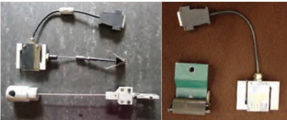
Figure 6 - Load cell and grips
