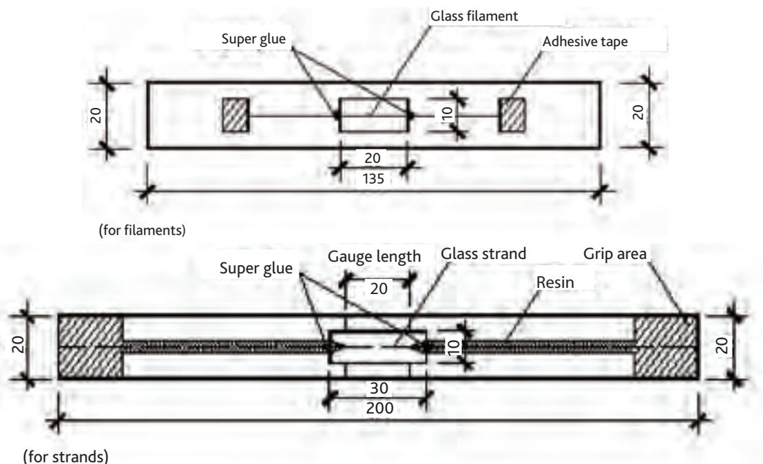
Figure 4 - Mounting tab dimension and specimen mounting method
