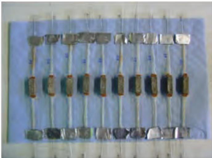
Figure 8 - Finished specimens
